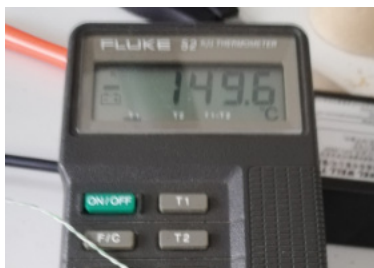
Fig. 2: Real ambient conditions of the valve in the WB workspace Temperature measurement
